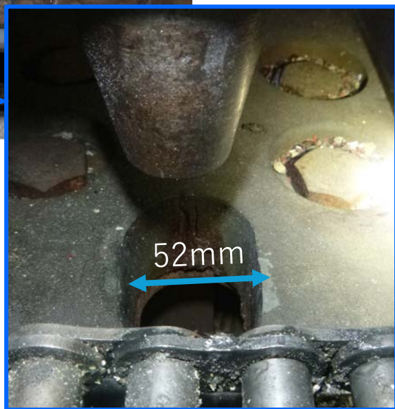
Stow pin ( \phi 46mm)
